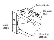
Fig. 4 Attaching a Read.me switch to bracket and tie rod
